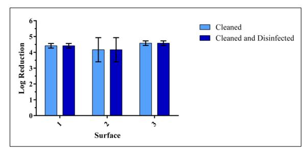
Figure 39. Log Reduction Values for Cleaned and Disinfected 3M<sup>TM</sup> Air Mate PAPRs.
