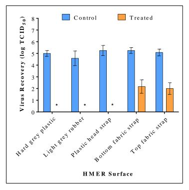
Figure 51. Viable influenza recovered from triplicate 3M 6200 respirators treated with low washer/disinfector conditions. (\* = below detection limit)
