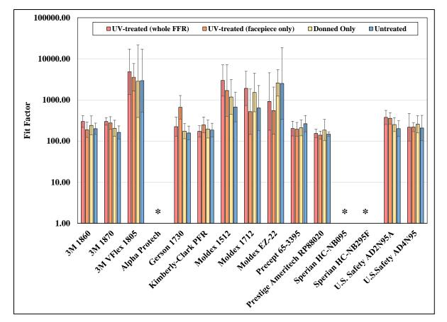
Figure 18. Mean Fit Test Data for 15 FFR Models Treated with 10 UVGI Cycles. (Note: \* indicates FF > 100 was not achieved)
