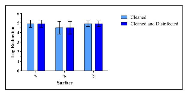
Figure 42. Log Reduction Values for Cleaned and Disinfected 3M<sup>TM</sup> Hoods.
