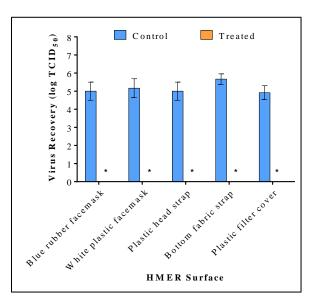
Figure 56. Viable influenza recovered from triplicate Sperian Survivair respirators treated with medium washer/disinfector conditions. (\* = below detection limit)
