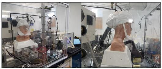
Figure 49. PAPR testing using medium static advanced headform.
