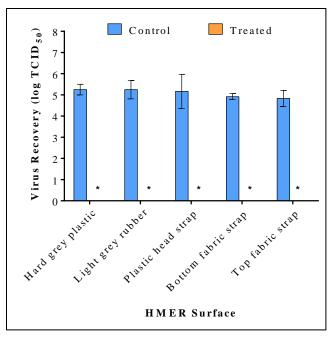
Figure 52. Viable influenza recovered from triplicate 3M 6200 respirators treated with medium washer/disinfector conditions. (\* = below detection limit)
