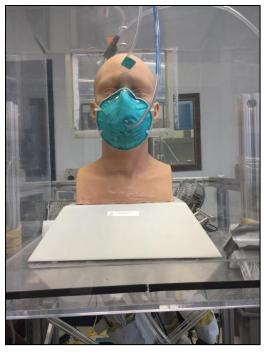
Figure 10. Fit Test Static Headform During Fit Test.
