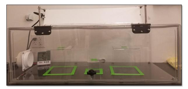
Figure 30. UV Exposure Device.
