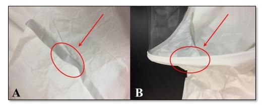
Figure 50. A) Tychem-Tychem seam, B) Tychem-visor seam.
