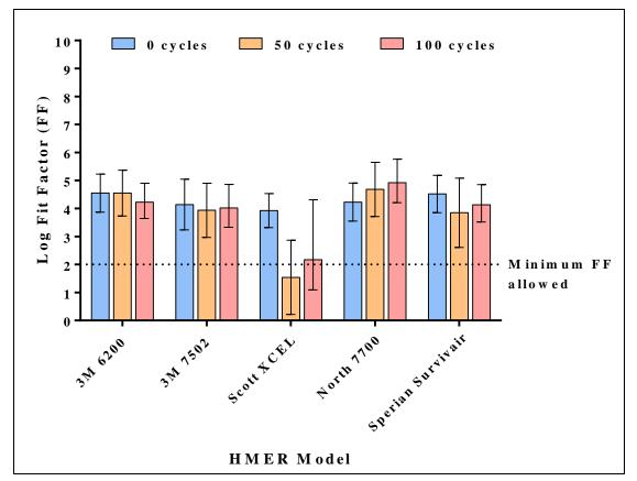
Figure 59. Fit test data of five HMER models treated with washer-disinfector using medium conditions.
