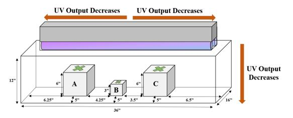
Figure 31. UV Exposure Device Layout.
