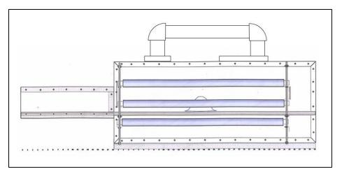
Figure 6. UVGI Device – Sagittal Cross-Section.
