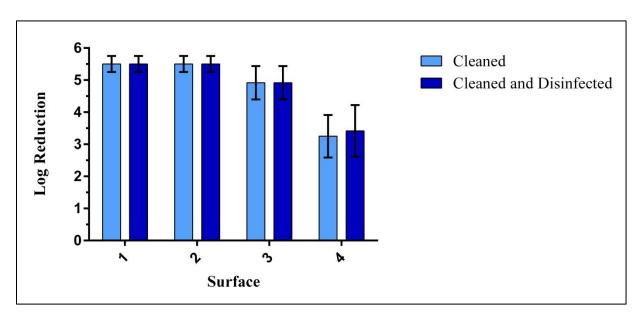
Figure 36. Log Reduction Values for Cleaned and Disinfected North<sup>®</sup> by Honeywell 7700 HMERs.
