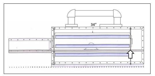
Figure 8. UV Radiometer Location within UVGI Chamber.
