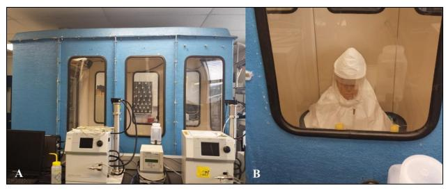
Figure 44. A) Large fit testing chamber, B) PAPR donned on headform in chamber.
