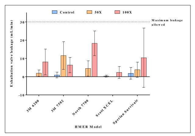
Figure 60. Exhalation valve leakage of five HMER models treated with washer-disinfector using medium conditions.
