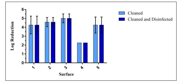
Figure 35. Log Reduction Values for Cleaned and Disinfected 3M<sup>TM</sup> 7500 HMERs.
